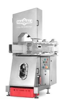
The MULTISPLITTER SAW with splitting conveyor has a special design with multiple saws that are working in parallel providing longitudinal cuts.
